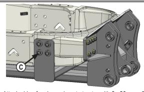
**5.** Attach side of undercarriage to tractor with 8 - 20mm x 50mm bolts and 8 - 3/4" x 3/8" thick heavy washers **(C)**.
