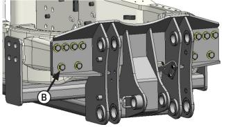
**4.** Raise undercarriage and attach front of undercarrige to tractor with 12 - 20mm x 70mm bolts and 12 - 3/4" flat washers **(B)**.
