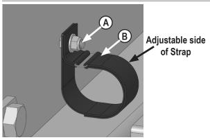
Attach a velcro hose strap on every bolt along undercarriage with a 3/8" flange nyloc nut (A). Assemble strap with the metal loop on bottom side as shown (B). Keep straps open.
