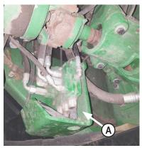
2. Locate steering hydraulics behind right axle and remove valve bracket bolts and move valve and bracket out of the way to gain access to 3 holes (A).
