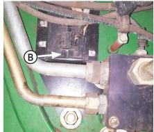
**3.** If applicable, remove hardware from drive shaft sensor controller **(B)** on left inside frame of tractor. The sensor will be reattached with new hardware in Step #12-13.
