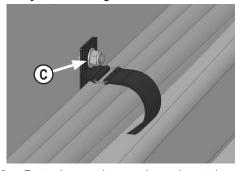
Route hoses along undercarriage tubes and secure with velcro straps (C).
