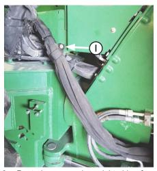
**8.** Route hoses up along right side of rear frame and group hoses together with a velcro strap. Attach velcro strap to the PTO shield with original hardware (I).
