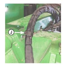
**9.** Use a velcro strap to group hoses together and attach to the PTO shield with 1 - 5/16" x 1" bolt and 1 - 5/16" flat washer (J).
