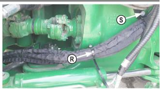
5. Route hoses upward through tractor. Staying away from the driveshaft. Group hoses together with zip ties (R). Remove bottom bolt from guard and bolt on velcro strap with a fender washer and original bolt. Secure hoses with strap (S).
