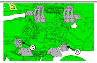
NOTE The orientation of left and right front brackets is important. Install the brackets as shown above.
