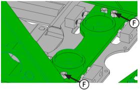
**11.** Attach rear of undercarriage vertically to cross member on tractor frame behind rear axle with 4 - 7/8" x 3" bolts, 8 - 7/8" hardened flat washers, and 4 - 7/8" nuts (**F**).
