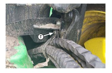
Secure hoses with a velcro strap (T) above rear axle with original hardware.
