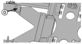
26. Install hose guard plate to rear of undercarriage with 4 - 1/2" x 1" carriage bolts, 4 - 1/2" washers and 4 - 1/2" nuts (O). Install bolts from top. Torque 1/2" nuts to 78 ft-lbs.
