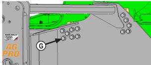
NOTE: Follow Steps #12-16 for left side. After Step #16, tighten bolts until they are snug. If necessary, add more shims on right side until a gap of 1/16" or less is on right side. Proceed with Step #12-16 for right side.
