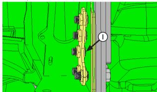
16. Place controller from Step #14 on bolts and thread a 3/4" flange nut on top 4 bolts from Step #15. Attach nut plate to bottom bolt and line up top hex nuts to fit in nut plate (I). Note orientation of flange nuts.
