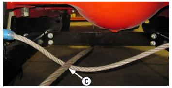
**3.** Route the cable underneath the undercarriage, then over the cable support and under the undercarriage on the right side **(C)**.
