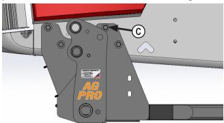
7. Install 8 - 20mm x 70mm bolts, 8 - 3/4" ID thick washers, shims if necessary, 8 - 3/4" flat washers, and 8 - 20mm nuts into the front side holes of the undercarriage and tractor frame (**C**).
