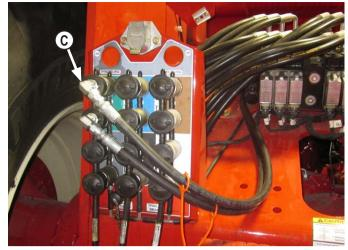
**5.** After installing the male couplers, plug each set into a set of rear SCV's **(C)**.
