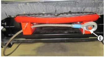
**5.** Finish routing the cable under the lift frame and up over the cable bracket. Attach to the bracket with the original hardware **(E)**.
