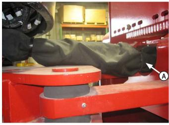
**2.** After routing the hoses through the undercarriage, route in the same location as the tractor's hoses **(A)**. Replace zip ties if you run the hoses in the tractor's original hose cordura.
