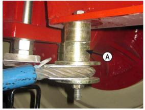
1. Add 2 spacers in between the cable holder and the tractor frame by the front tires. Use a 5/8" x 6" bolt (PN: 16-20200), 2 - 5/8" washers (PN: 57-20746) and a 5/8" top lock nut (PN: 70-20646) on each side (A).
