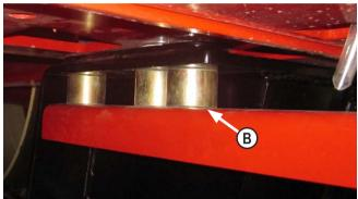
**2.** Install the front cable support bracket at the front of the undercarriage. Install with 3 spacers on each side in between the undercarriage and the bracket. Use 3 - 20mm x 120mm (PN: 16-2489) to install the bracket and undercarriage. Use the same washers and nuts from Step #8 on Page 3 (**B**).
