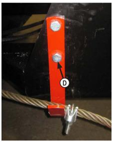
**4.** Install the original bracket to the side of the undercarriage with  $2 - 3/4^{\circ} \times 2^{\circ}$  bolts (PN: 16-20218) and  $2 - 3/4^{\circ}$  nuts (PN: 70-20607) **(D)**. Cable clamp is installed in Step #6.
