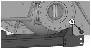
5. Raise the rear of the undercarriage and attach the rear bracket to the frame of the tractor behind the front axle with 2- 20mm x 70mm bolts, 4 - 3/4" ID thick washers, and 2 - 20mm nuts (B).
