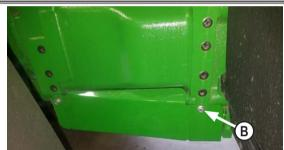
Remove cover on left side of tractor in front of fuel tank (B). 3.
